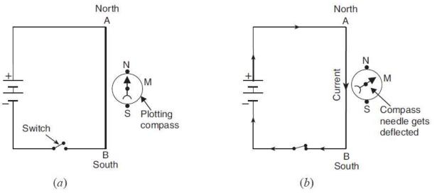
the deflection of compass needle by the current carrying wire in the above experiment shows that an electric current produces a magnetic field around it.
