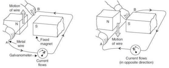
1. Let us move the wire AB upwards rapidly between the poles of the horseshoe magnet. When the wire is moved up, there is a deflection in the galvanometer pointer showing that a current is produced in the wire AB momentarily which causes the deflection in galvanometer. The deflection lasts only while the wire is in motion. Thus, as the wire is moved up through the magnetic field, an electric current is produced in it.
