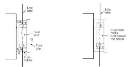
Fuses are used to protect the individual domestic electrical appliances from damage which may be caused due to excessive current flow through them.
