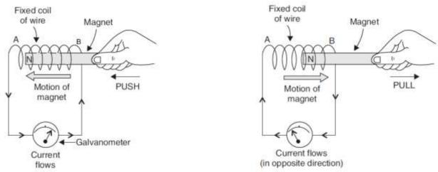
When a bar magnet is moved quickly into a fixed coil of wire AB, then a current is produced in the coil. This current causes a deflection in the galvanometer pointer. Similarly, when the magnet is moved out quickly from inside the coil, even then a current is produced in the coil.
