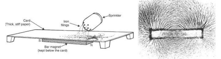
iron filings show the shape of magnetic field produced by a bar magnet by aligning themselves with the magnetic field lines.
