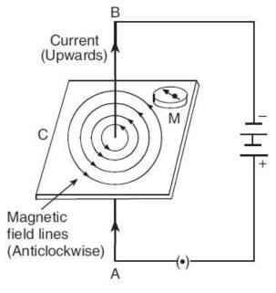
Field - Circular Direction of current - Right Hand Thumb Rule/ Maxwell's Corkcrew rule
