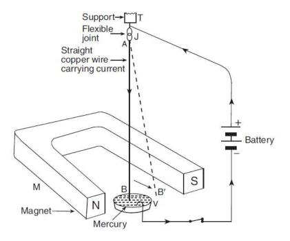
The direction of force acting on a current-carrying wire placed in a magnetic field is (i) perpendicular to the direction of current, and (ii) perpendicular to the direction of magnetic field. **Note** - the direction of force on a current-carrying conductor placed in a magnetic field can be reversed by reversing the direction of current flowing in the conductor.
