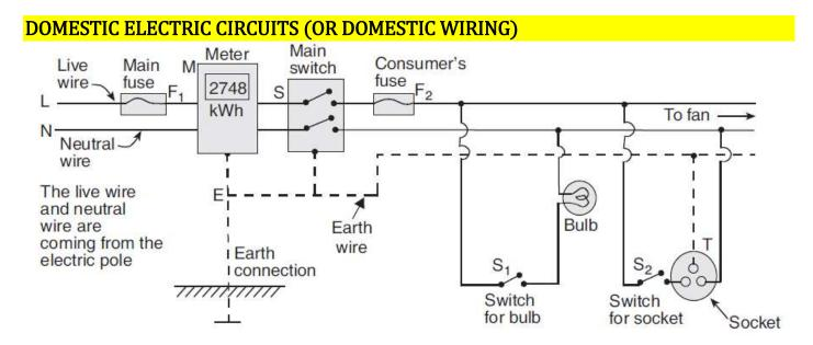
**Note -** In order to distinguish between the live wire, neutral wire and earth wire, the wire having red plastic covering is made live wire, the wire having black plastic covering is made neutral wire, and the wire having green plastic covering is made earth wire.
