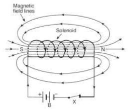
**Field -** similar to bar magnet **Direction of current -** Clock Face Rule
