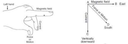
According to Fleming's left-hand rule : Hold the forefinger, the centre finger and the thumb of your left hand at right angles to one another. Adjust your hand in such a way that the forefinger points in the direction of magnetic field and the centre finger points in the direction of current, then the direction in which thumb points, gives the direction of force acting on the conductor.
